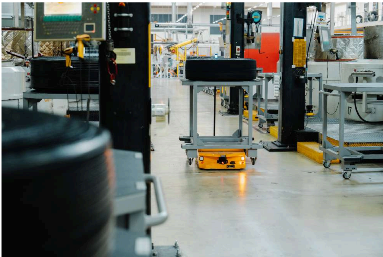
An autonomous mobile robot, directly connected to Continental's digital order system, transports a tire to the curing press using a trolley.
